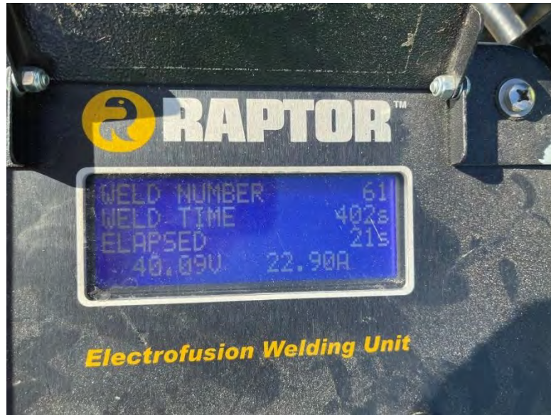
Photo 3: Raptor welding equipment shown during the welding sequence.
