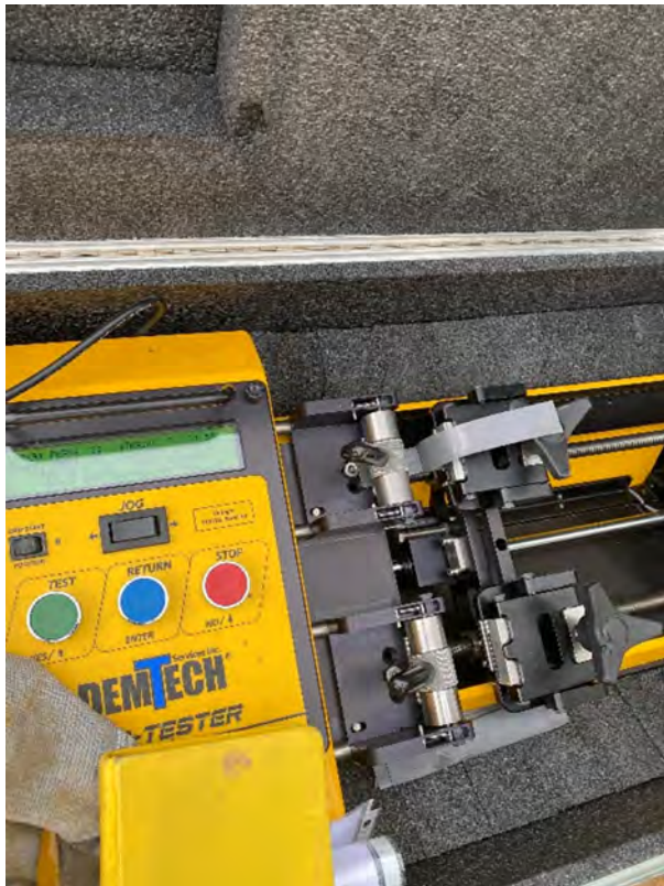
Photo 4: Field tests on fusion trial weld.
