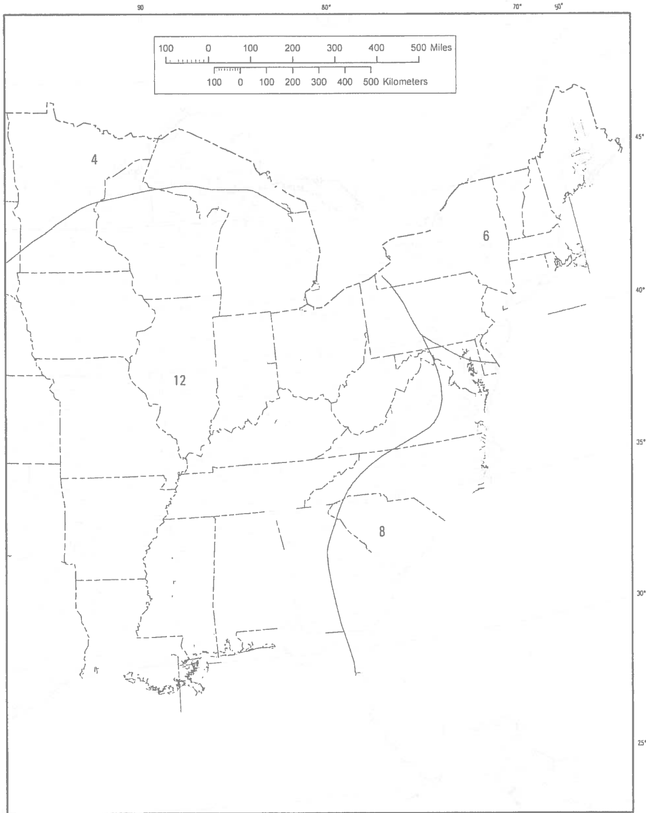
Figure 22-12 (continued) Mapped Long-Period Transition Period, T_1 (s), for the Conterminous United States.
