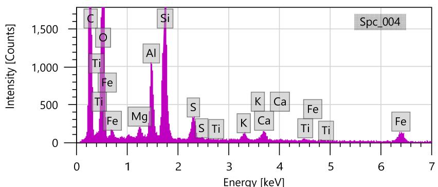
Lignite. Backscattered electron micrographs show the sample at 100X, 1,100X, and 1,500X. EDS spectrum at bottom is an area scan of the region shown in top right micrograph. Bright particles are mostly quartz and feldspar. Major peaks for carbon, oxygen, silicon, and aluminum suggest coal and clay.
