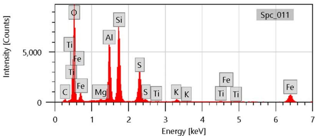
Sample VAP B3 50-55. Backscattered electron micrographs show the sample at 250X, 500X, 1000X, and 3000X. EDS spectrum at bottom is an area scan of the region shown at 3000X. Bright particles are mostly pyrite (framboid in bottom left micrograph); occasional particles of Fe-Ti oxide are detected. Major peaks for oxygen, silicon, and aluminum suggest clay. Large blocky particles are mostly quartz, feldspar, and clay.
