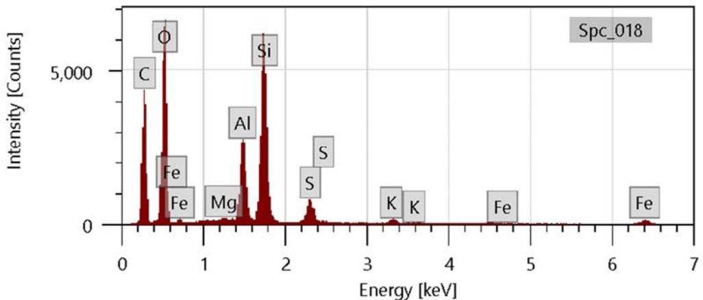
Sample VAP B3 40-45. Backscattered electron micrographs show the sample at 100X, 250X, 500X, and 3000X. EDS spectrum at bottom is an area scan of the region shown at 500X. Bright particles are pyrite (framboid in bottom right micrograph). Major peaks for carbon, oxygen, silicon, and aluminum suggest coal and clay.
